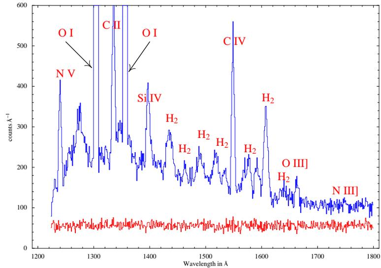
Fig. 2. Simulated HUBE Far Ultraviolet Spectrograph (FUVS) Observation: a 3600-s integration of the diffuse UV background at high galactic latitudes. The lower line (near zero) is the contribution of detector internal background to the observed signal. Molecular hydrogen emission, high-ionization line emission, and continuum are all detected easily. Geocoronal emissions, at O I 1304 and 1356 Å, are easily removed.
